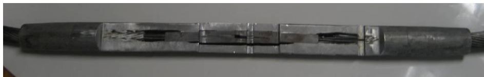
Image 2. Sectioned ACSR MidSpan Joint Showing pressed Steel Inner Sleeve
