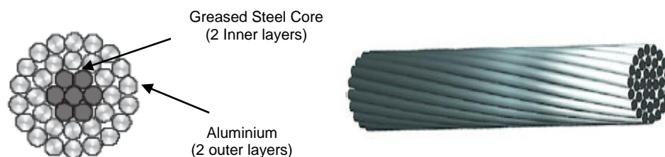
Figure 1. Typical ACSR Conductor
