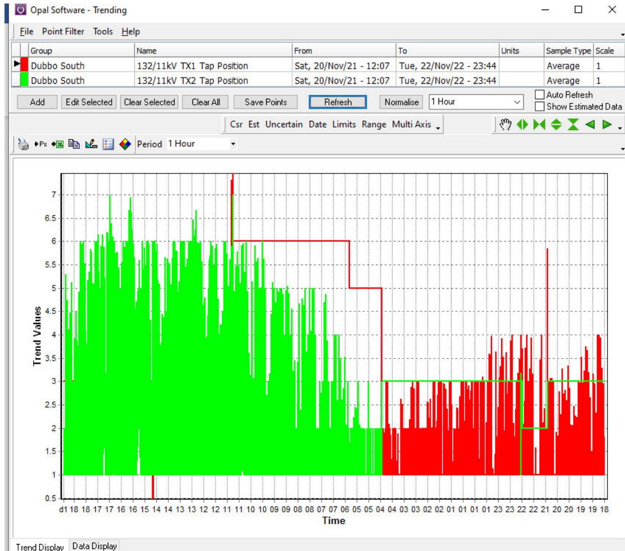
Figure 5: Dubbo South 132/11kV Transformer Tap Position Nov 2021 to Nov 2022
