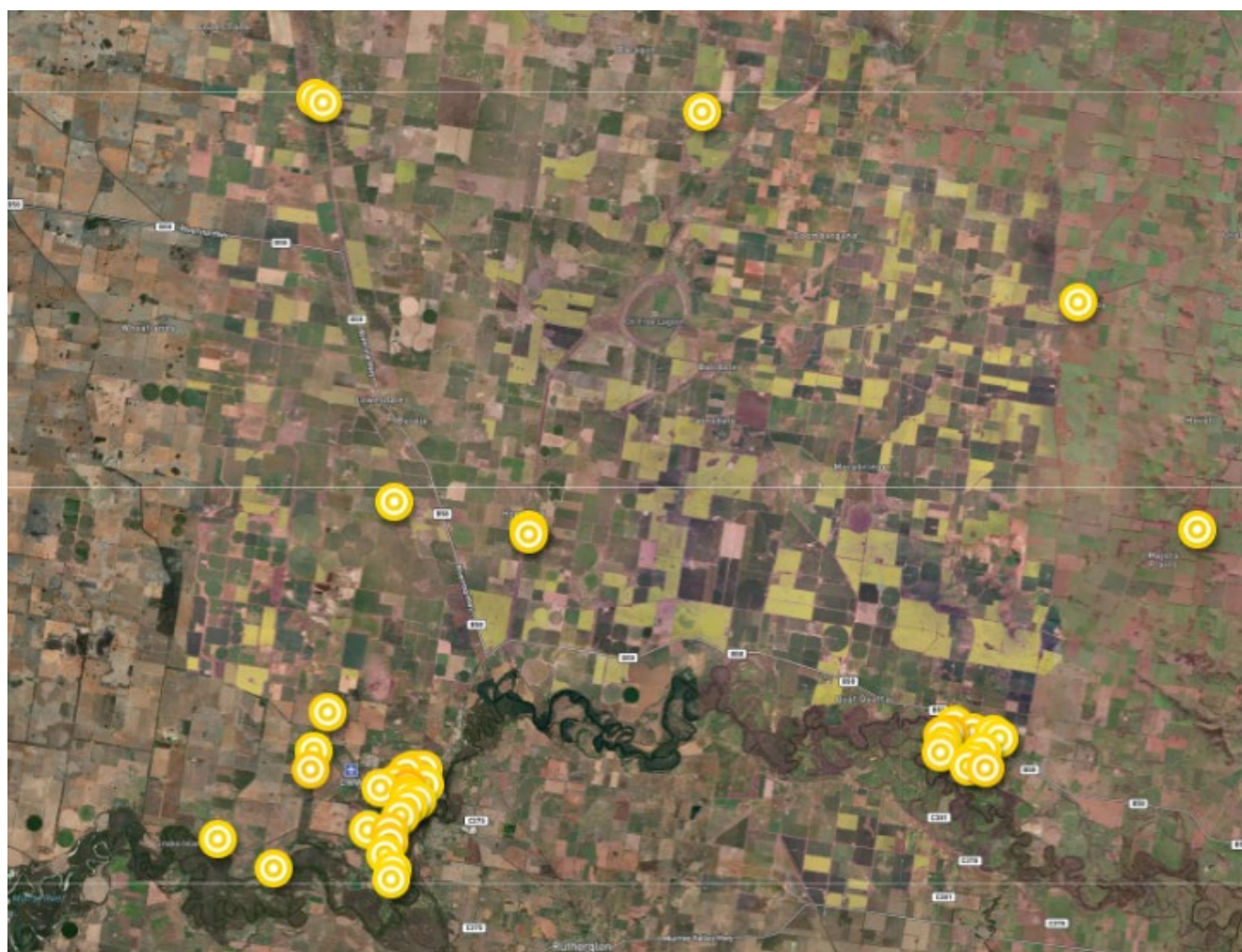
Figure 4: High Voltage Issues Detected by Smart Meters on Corowa Network
