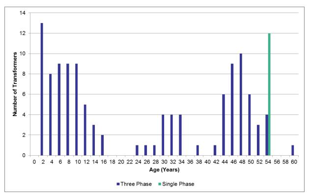
Figure 5 – Service Age of Connection Transformers
