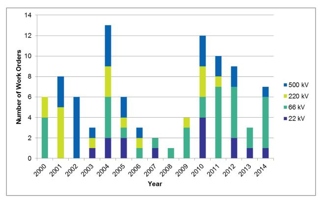
Figure 27 – Work order history by oil filled reactor voltage
