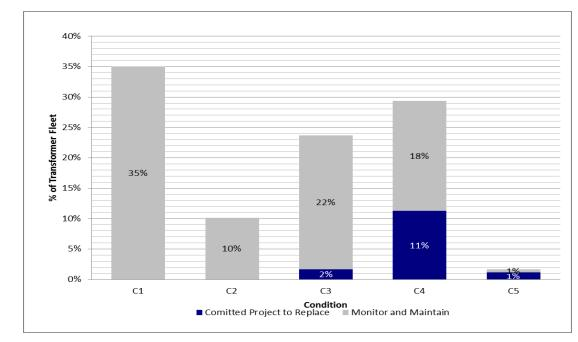
Figure 14 shows the percentage of transformers held in each overall weighted condition score.
