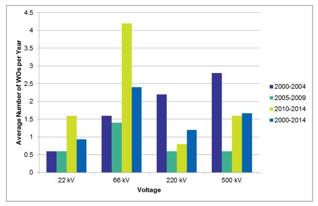
Figure 29 – Average number of work orders per year during different time periods per voltage
