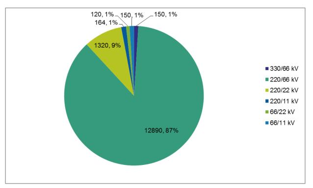
Figure 2 – Installed Capacity (MVA & as a percentage) of Connection Transformers by Voltage Ratio
