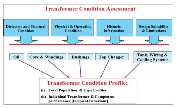
Figure 8 – Flow Chart for objective Condition Assessment Methodology
