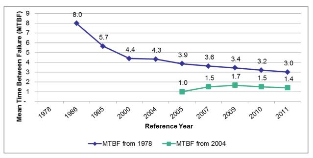
Figure 23 – Mean Time Between Major Transformer Failure (MTBF)
