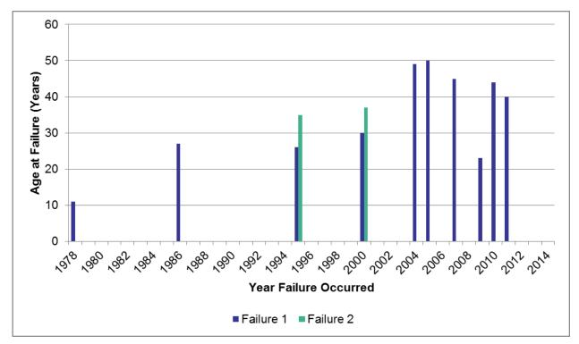
Figure 22 – Year and Service age at time of Major Transformer Failures
