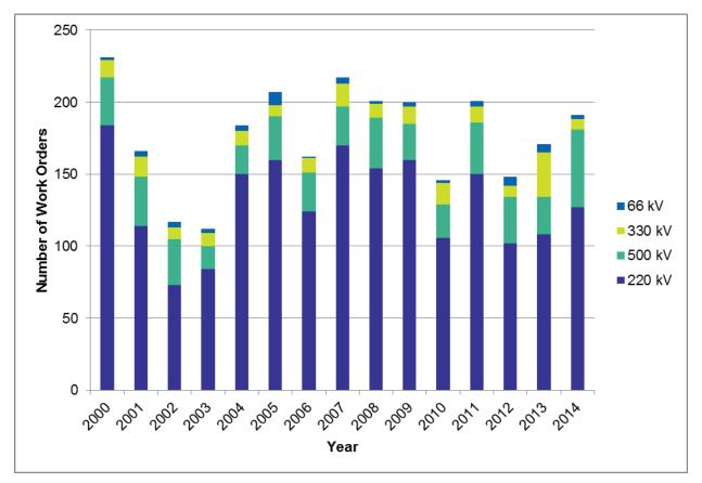
Figure 24 – Unplanned transformer work orders 2000 to 2014
