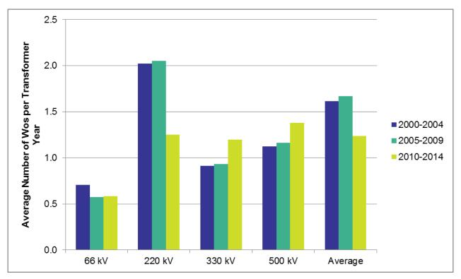
Figure 25 - Average number of unplanned work orders per transformer year
