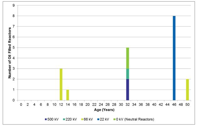
Figure 7 – Service Age of Oil Filled Reactors
