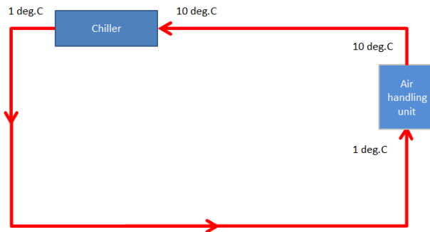
Figure 6.1: Typical air-conditioning cooling cycle
