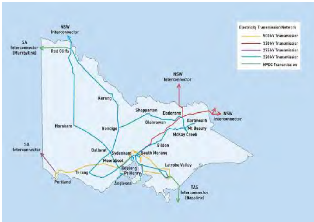
Figure 5: Victorian Electricity Transmission Network
