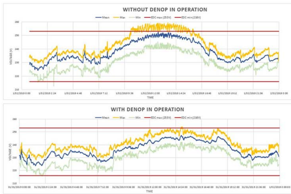
Figure 14: Voltage traces at customer site with and without DENOP in operation
