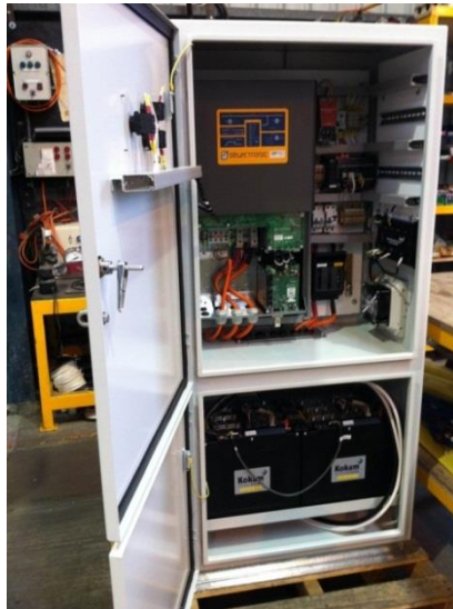
Figure 5 - Example residential battery storage system with 6.6kWh storage
