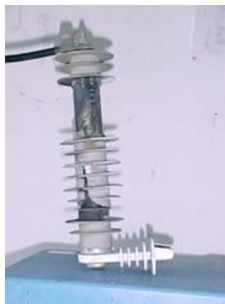
Figure 11 - Failure of Polymeric Surge Arrester Housing
