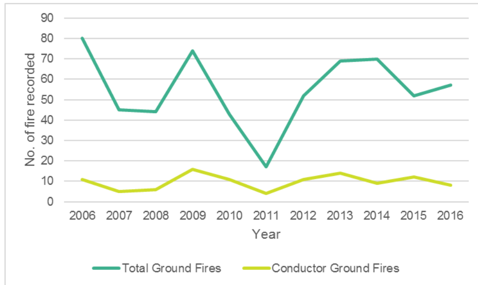
Figure 24 – Ground fires caused by conductor defects
