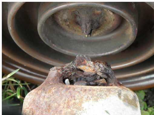
Figure 13 – Failed insulator string due to pin corrosion
