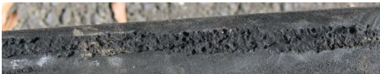
Figure 16 – Screen pitting of the insulation screen of NMS HV ABC caused by sheath arcing.
