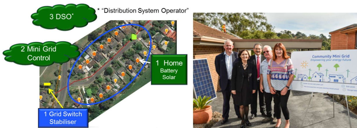
Figure 2 a) Site layout and key components of the Mini Grid, b) Official opening of the Mini Grid
