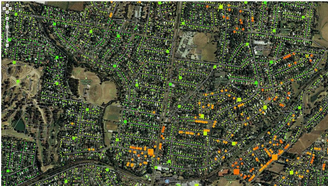
The above diagram shows one way in which smart meters are improving network operations. Voltage is monitored at an individual customer level in near
