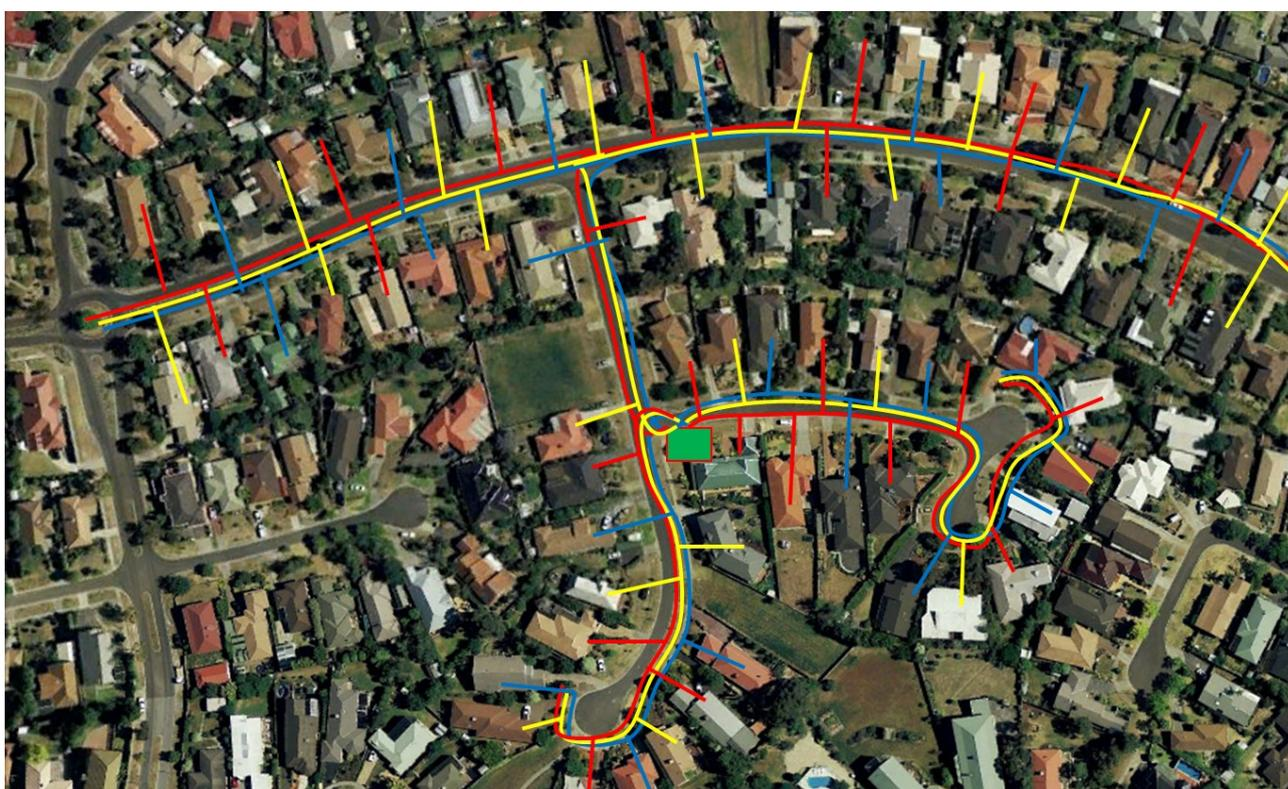
The above diagram shows how smart meters enable better network planning. The distribution substation transformer is shown as the green square in the centre. The coloured lines represent the low voltage electricity phase at each property.
