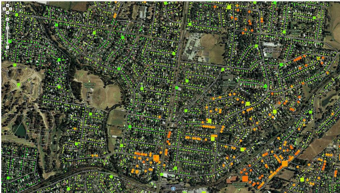
The above diagram shows one way in which smart meters are improving network operations. Voltage is monitored at an individual customer level in near real time, allowing better management of electricity supply and faster detection and location of outages, which means faster restoration of power.
