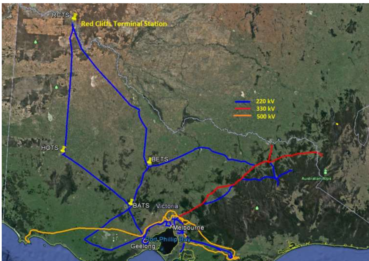
Figure 1 - Transmission network supplying Red Cliffs Terminal Station
