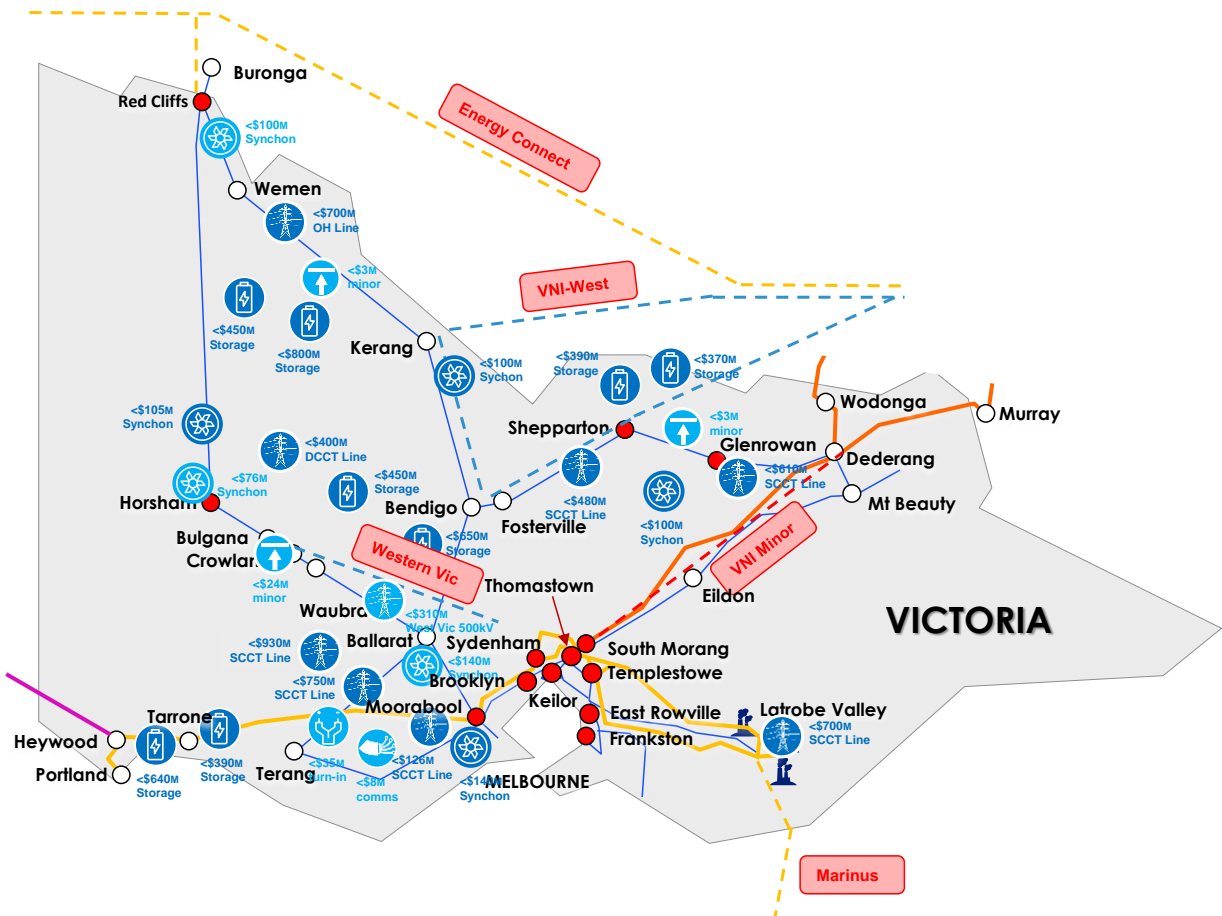
Figure 3-5: AusNet major station projects, ISP projects and REZ Development Plan (Stage 1 and Stage 2) projects
