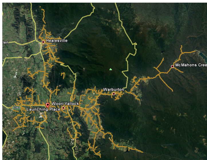
Figure 1-1: WYK 22kV overhead feeders shown above in orange.
