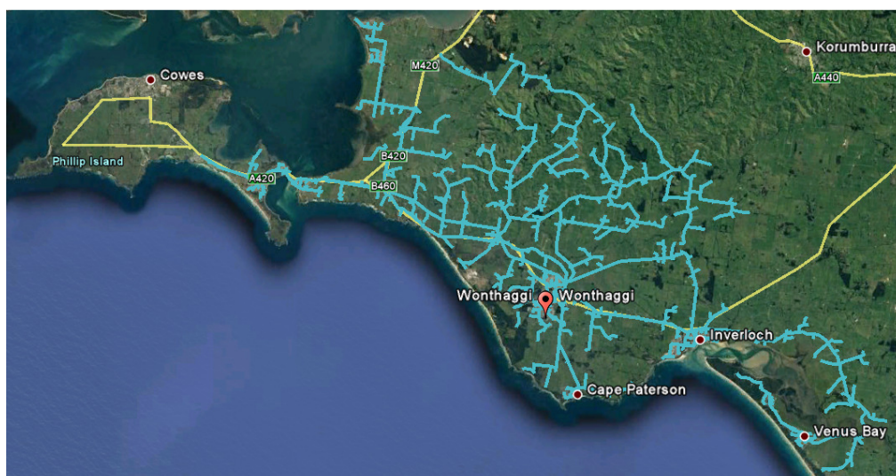
Figure 1-1: WGI 22kV feeders shown above in blue.
