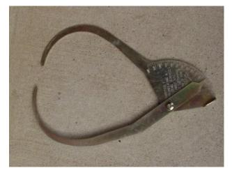
Figure 3.3.6: Outside Callipers Suitable for Measuring the Reduced Diameter of Poles. Range from 0–600mm
