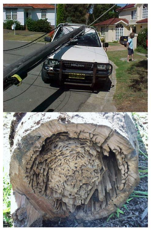
Figure 16 – The result of a breakdown failure of a wood pole caused by a combination of termite attack and rot
