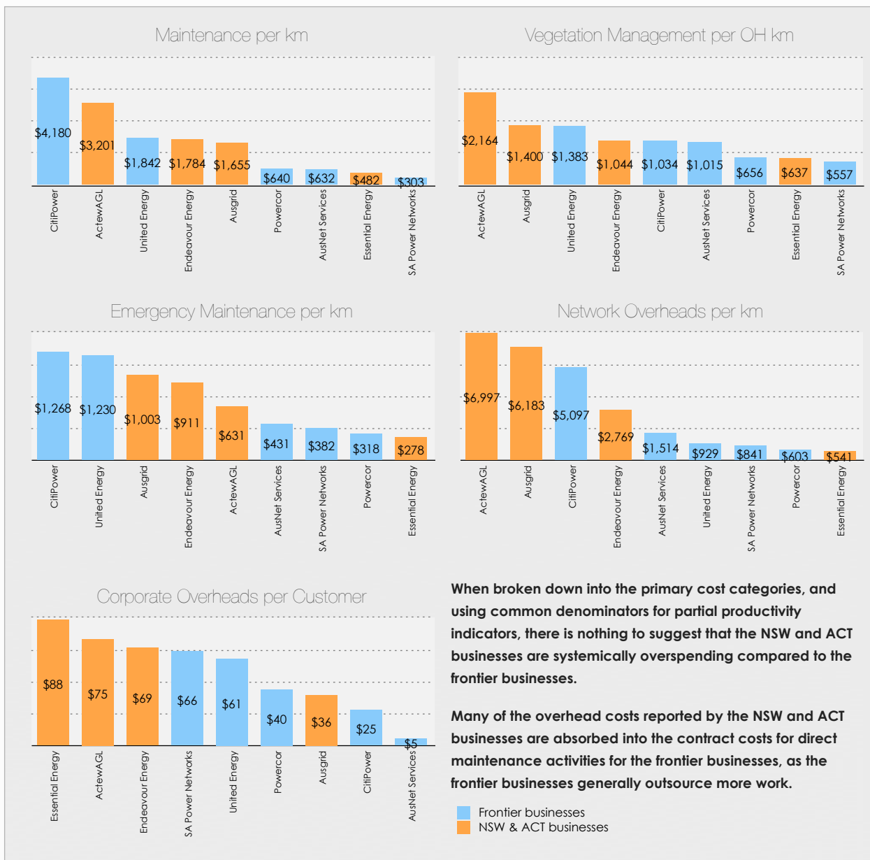
Exhibit 4.15: Partial productivity analysis demonstrates the practical issue with meeting the AER adjustments.
