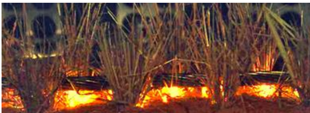
Distribution of conductor-soil arcs at instant of initial contact (16 amps, 19/3.25AAC conductor) 26
