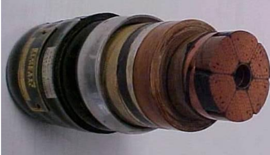
Figure 12. Typical 132KV single phase fluid filled cable
