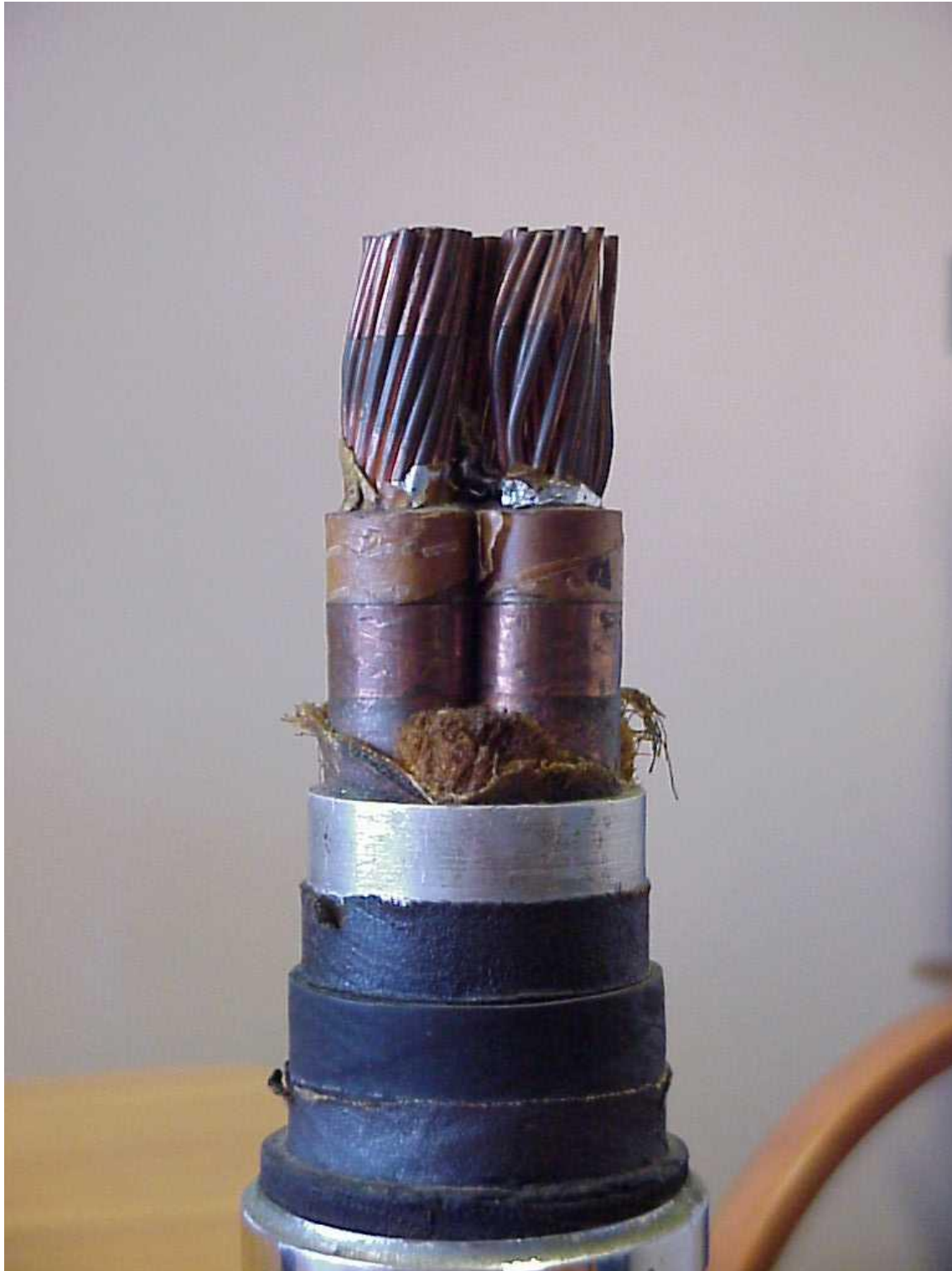
Figure 43. Typical 33kV three phase HSL cable
