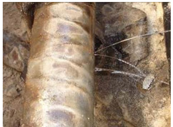
Figure 3. Leaking fluid filled cable
