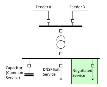
**Step 1:** The branches are Feeder A, Feeder B, DNSP Exit, Tie Transformer and Capacitor, the negotiated service branch is not considered as discussed above.
