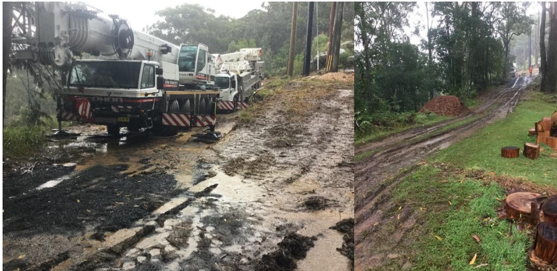
Figure 17: Site in Narara (customer property) where a 100T crane became bogged following sustained wet weather
