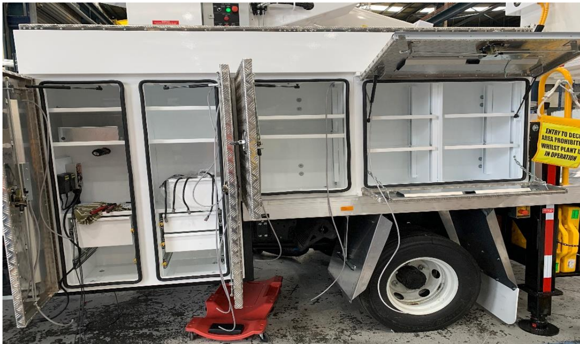
Figure 26: Standard equipment storage configuration for Nifty-Lift EWP during the fitout process
