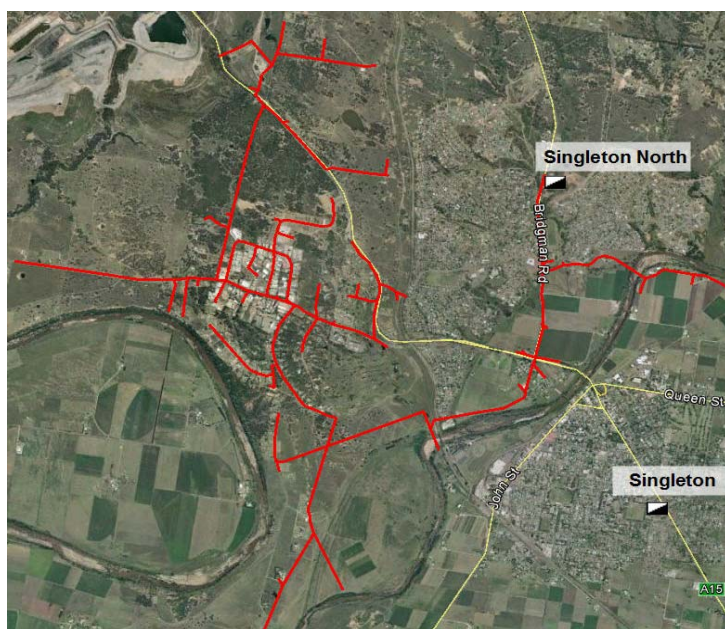
Figure E2 – A typical 11kV rural feeder
