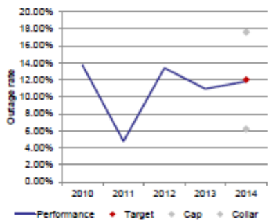
Figure 7.6: Unplanned outage circuit event rate – reactive plant (forced outages)
