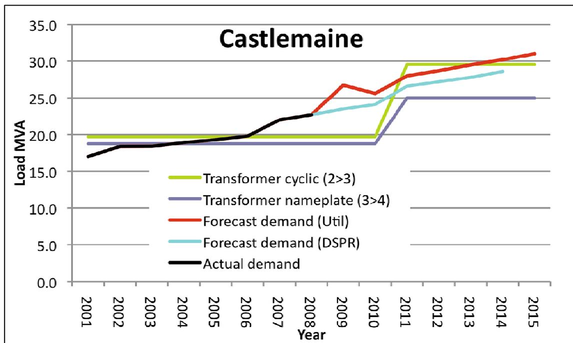
Based on Powercor's assessment of the firm (N-1) capacity of the substation, the substation load exceeds this by 22-37% in 2010. However, there is doubt concerning the validity of Powercor's firm capacity rating.
