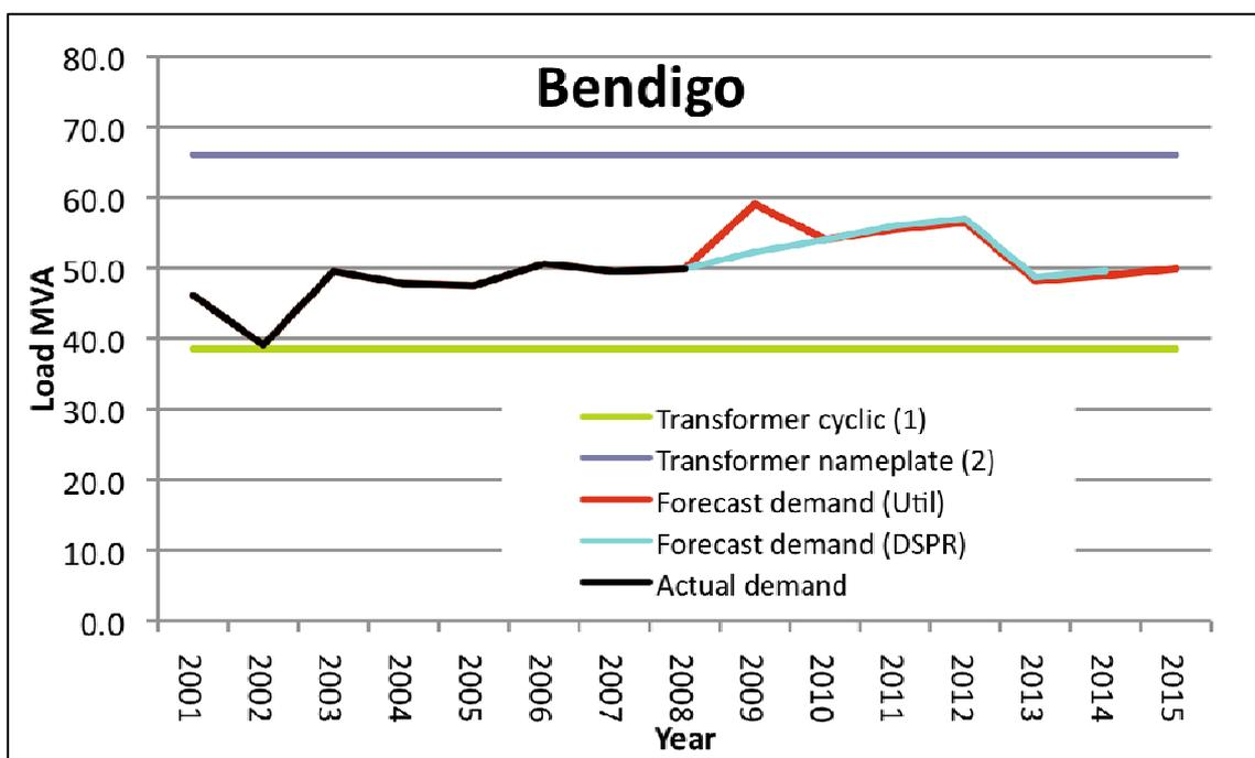
The summer cyclic rating of the Bendigo transformers is approximately 117% of the nameplate capacity. This level of emergency loading seems appropriate.
