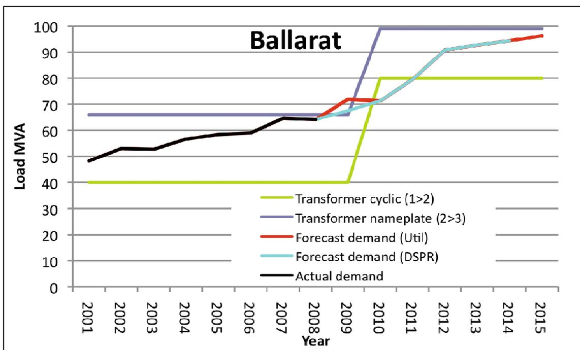
The summer cyclic rating of the Ballarat transformers is approximately 115% of the nameplate capacity, which is at within a feasible range.
