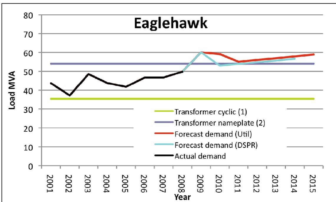
Based on Powercor's assessment of the firm (N-1) capacity of the substation of 35.4 MVA, the substation load would exceed this by 50% in 2010. However, as with Castlemaine, there is doubt concerning the validity of Powercor's firm capacity rating. A cyclic rating of approximately 130% of the transformer nameplate rating has been assigned by Powercor. A more reasonable assumption of 120% of the nameplate rating would yield a firm capacity of 32.4 MVA, which the load would exceed by 64%.
