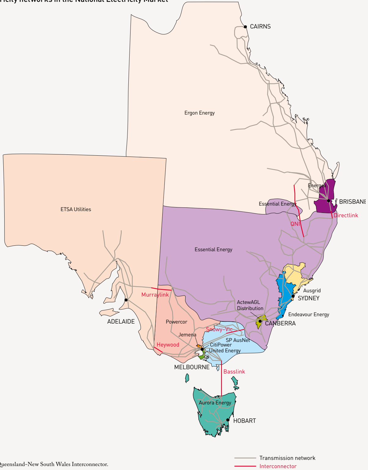
Figure 2.1 Electricity networks in the National Electricity Market
