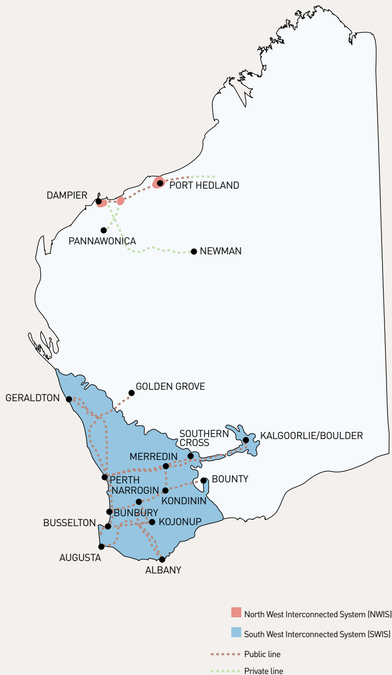
Figure 7.1 Electricity infrastructure map—Western Australia
