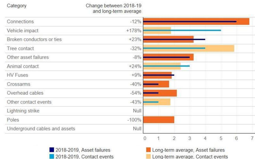
Figure 58 Incidents on the United Energy network resulting in ground fires
