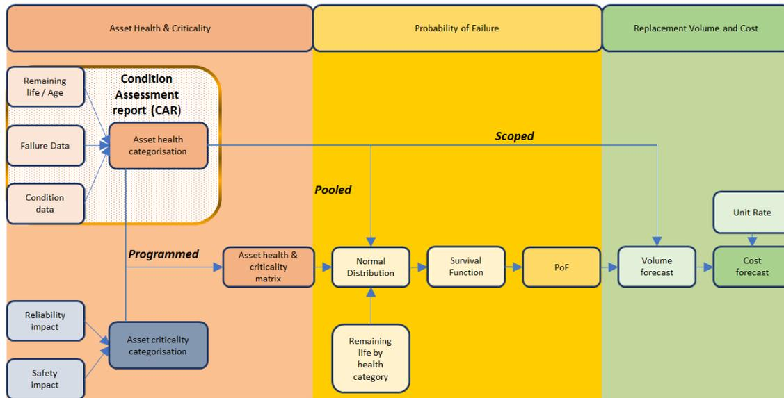
The output of the CAR is an assessment of remaining serviceable life before some form of intervention is required for the asset to continue to provide the service it was designed for. The information within the CAR is used as an input to determine the most effective asset class management plan and by definition the CAR **does not include a criticality assessment**.
