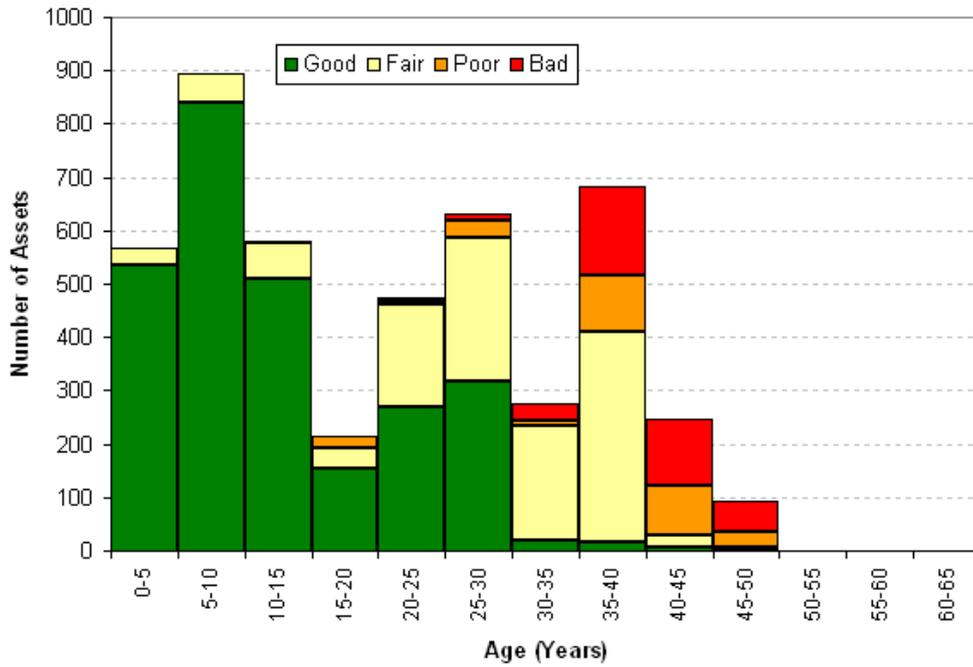
**Figure 7.38: Condition Profile of Current Transformers**
