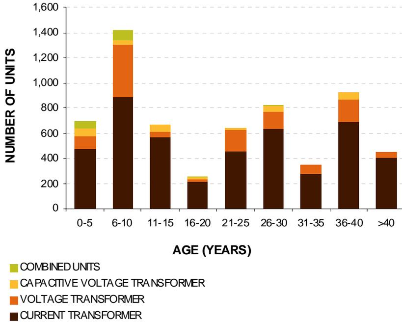
**Figure 7.36: Age Profile of Instrument Transformers**
