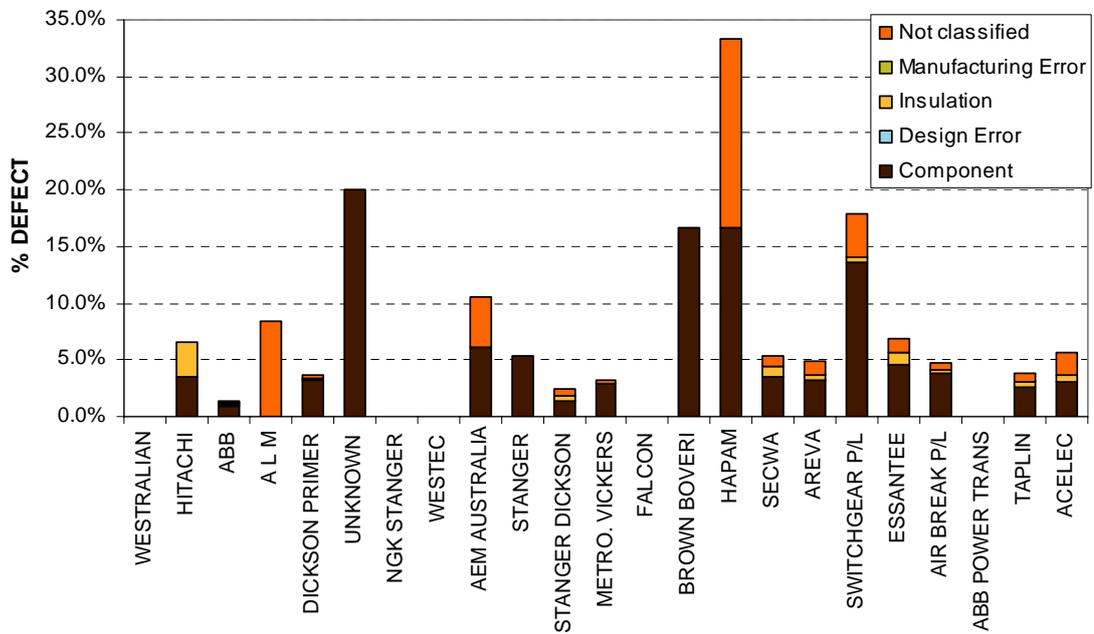
**Figure 7.30: Disconnectors failure mode and manufacturer**
