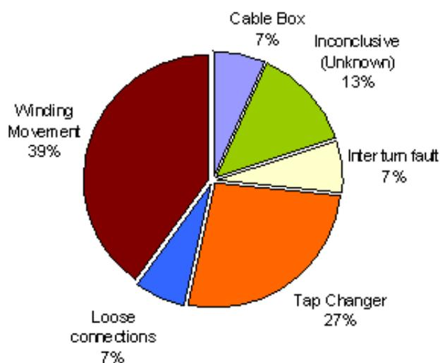
**Figure 7.4: Major transformer failures (since 1997)**
