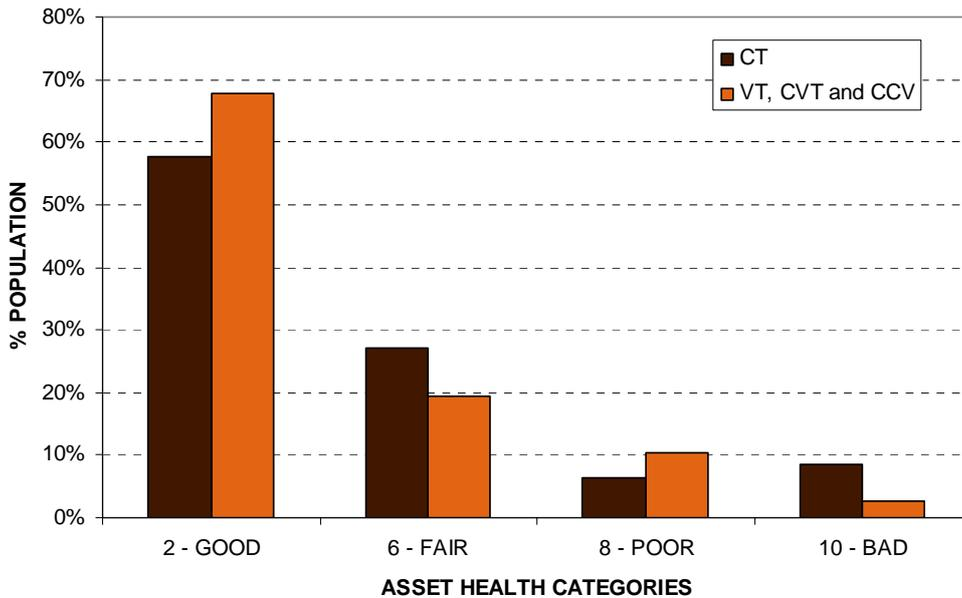
**Figure 7.37: Instrument transformer condition rating**
