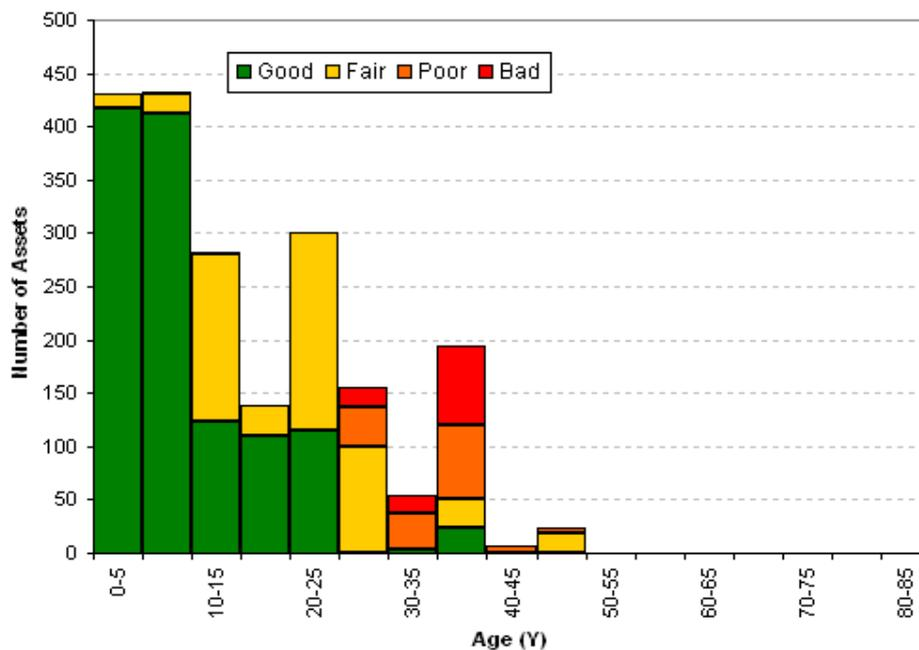
Figure 7.62: Transmission surge arrester condition profile
