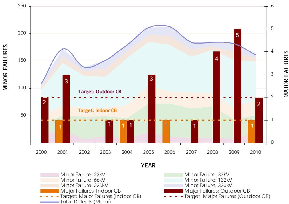
**Figure 7.27: Circuit breaker failure history**
