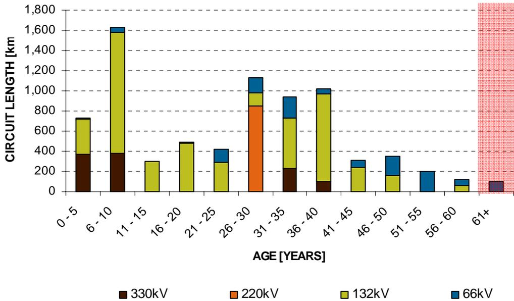
**Figure 7.9: Age profile of overall transmission overhead conductors**
