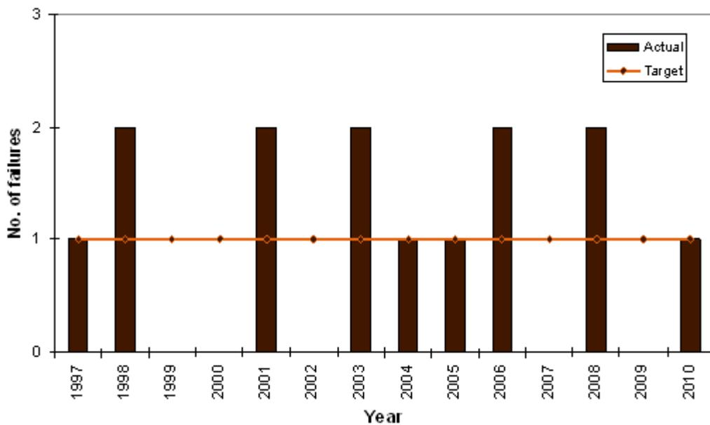
**Figure 7.7: Unplanned power transformer failures**
