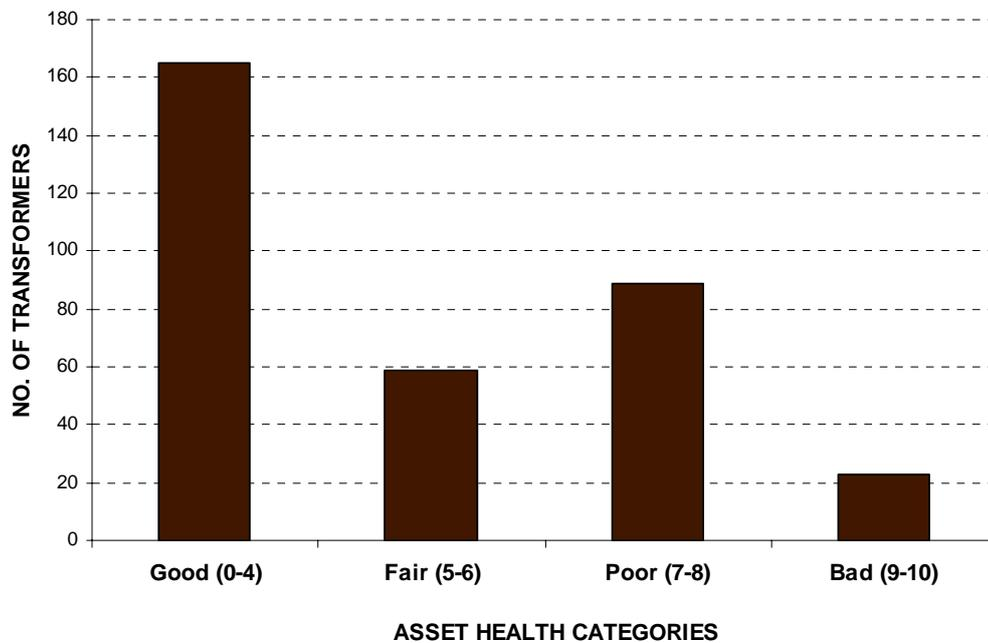
Figure 7.5: Power transformer condition rating
