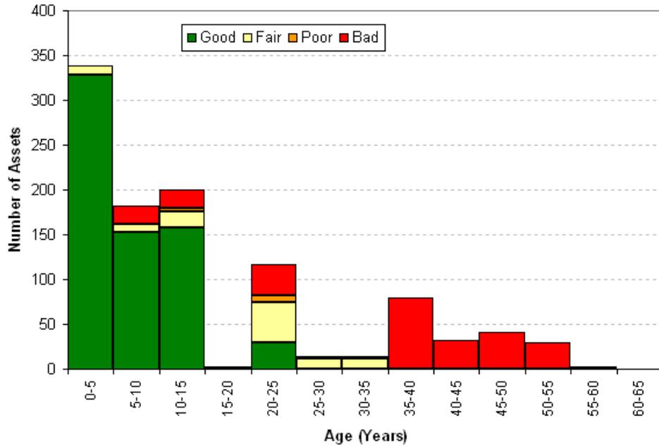
**Figure 7.24: Indoor Circuit breaker condition profile**
