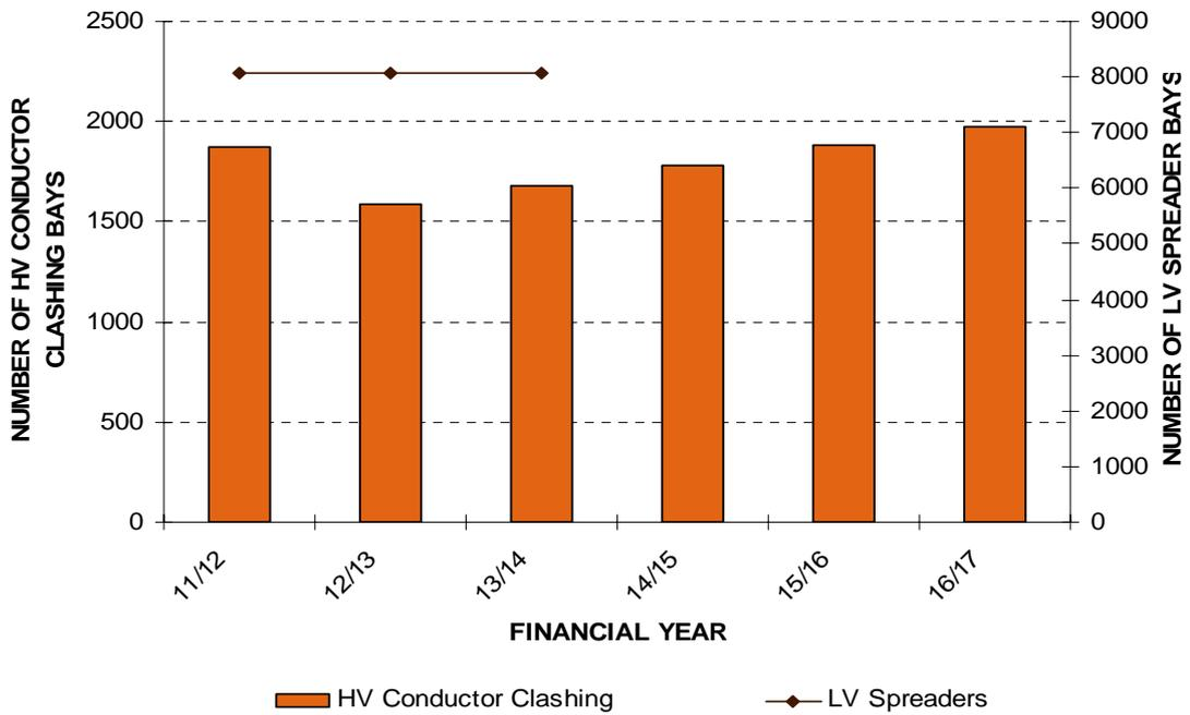
**Figure 7.12: Planned volumes for rectification under HV Conductor Clashing and LV Spreaders programs**
