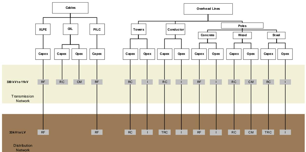
RF – Replace on failure, RC – Replace on Condition, TRC – Targeted Replacement based on Condition.
