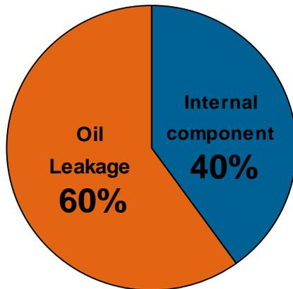
**Figure 7.21: Circuit breaker failure modes**
