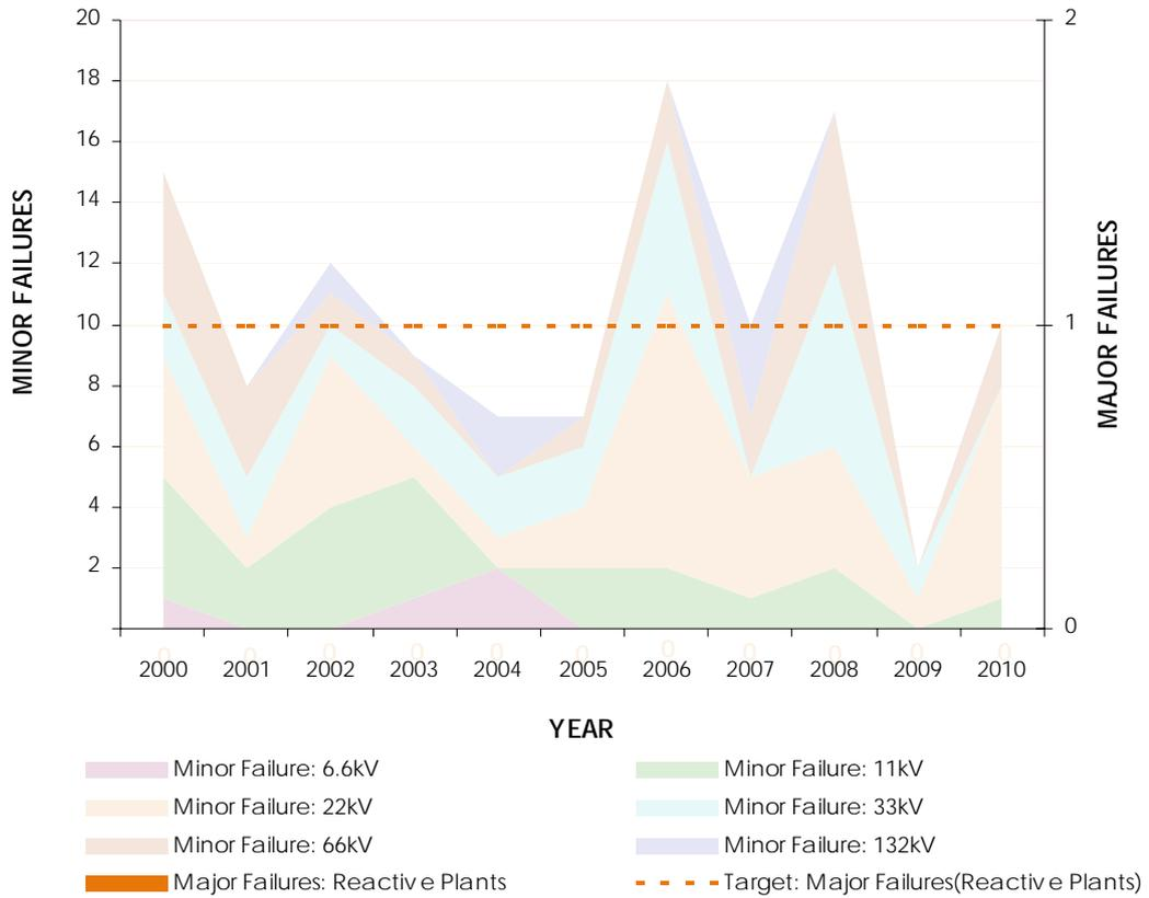
**Figure 7.43: Reactive plant failure comparison in the last 10 years**
