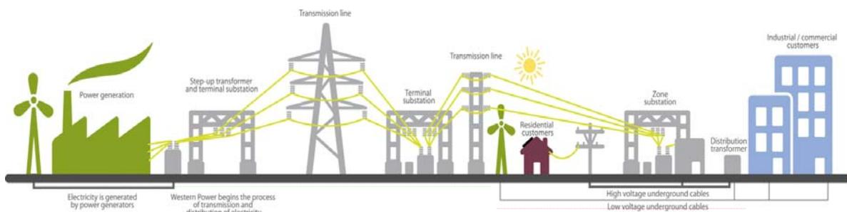
**Figure 1.3: How Western Power transports electricity (green is transmission and red is distribution)**
