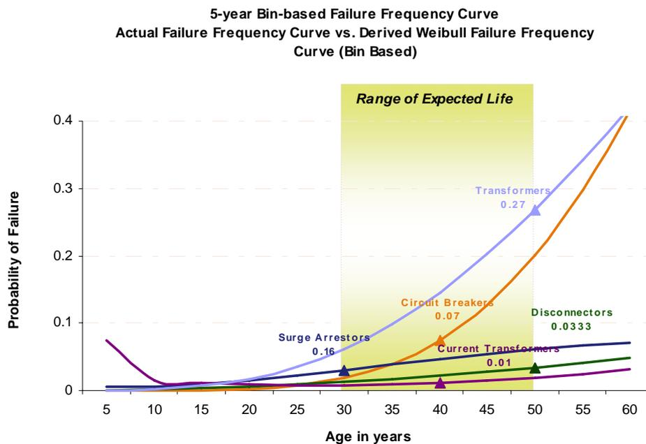
**Figure 4.8: Time to failure probability distribution curve**
