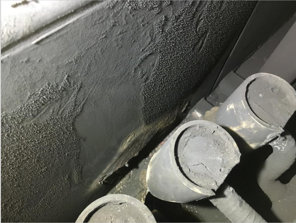
Figure 6 Damage and distortion of busbar chamber adjacent to failed circuit breaker busbar spouts
