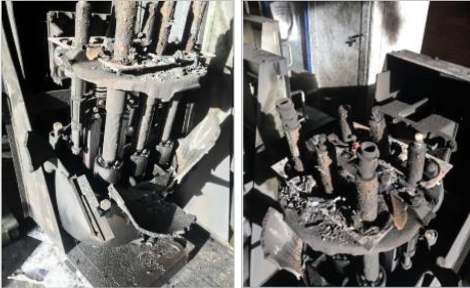
Figure 3 Extensive damage to B23 circuit breaker following a catastrophic failure
