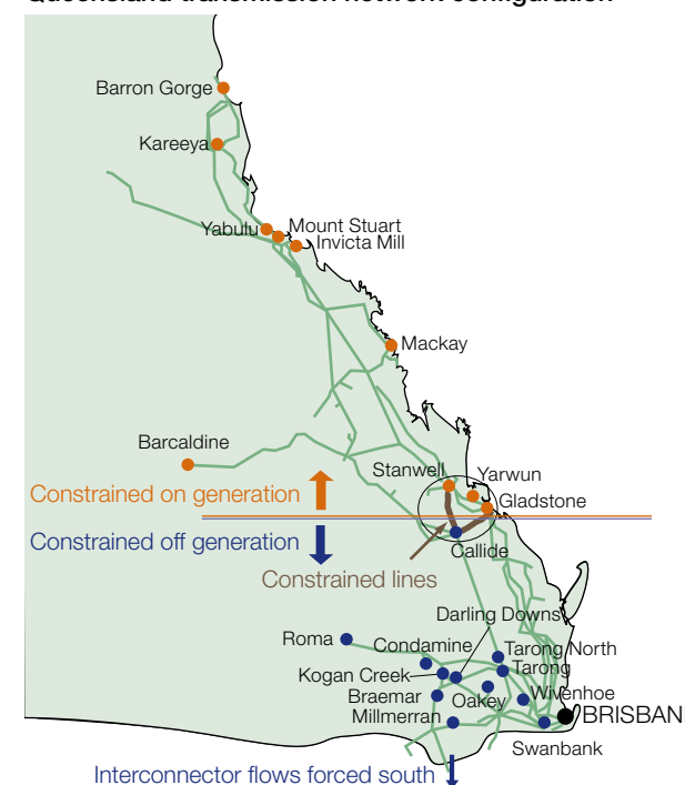
Figure 1.20 Queensland transmission network configuration
