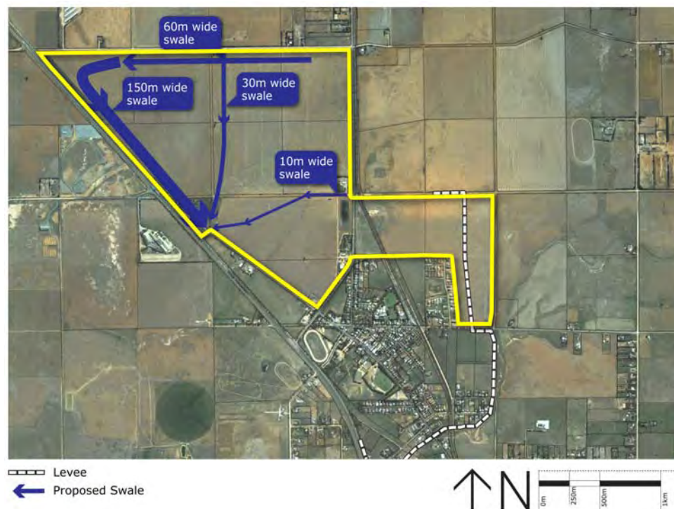
Figure 6.11 Location of Proposed Levee and Flood Diversion Channels
