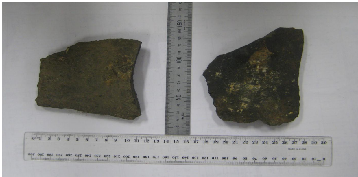
Figure 13-4: Parts of a 300mm diameter MP main
