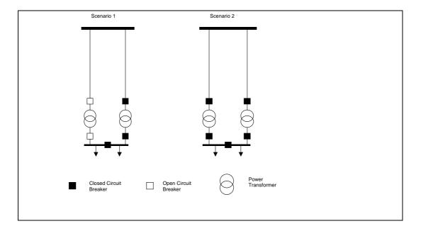
To properly protect the arrangement shown in Scenario 2, it is normal to provide some form of pilot wire, or "intertripping", arrangement. This arrangement ensures that for a fault on an incoming line, only the faulty line is disconnected and no interruption of customer load occurs.
