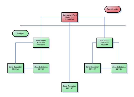
The diagram of the Energex supply network shows the zone substation load being supplied via bulk supply substations except in the case where direct transformation substations (110/11kV) are employed. DPA0601 is the 110/33kV bulk supply substation capacity to a meshed network supplying the 33/11kV zone substations
