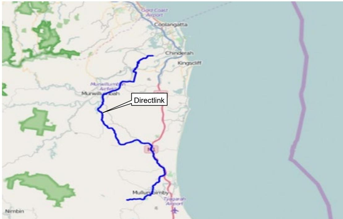
Directlink comprises six AC/DC converter stations (three at each end) and the six cables (three pairs) that link them, making up three circuits of 60 MW each. It is made up of both primary equipment (the major components operating at high voltage) and secondary equipment (necessary for the operation of the primary equipment).
