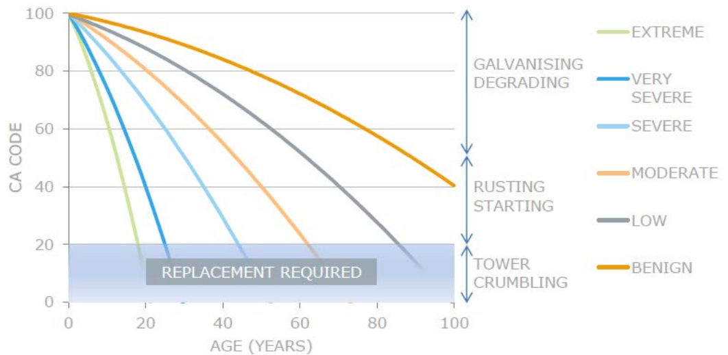
Figure 15: Tower steel degradation curves for unpainted towers
