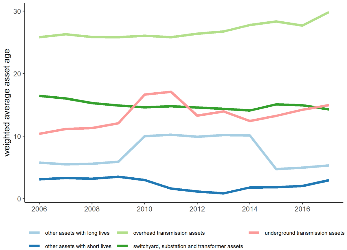
Figure B.2: NEM wide average asset age for transmission assets: Overhead assets have gotten older, substation and transformer assets have gotten younger
