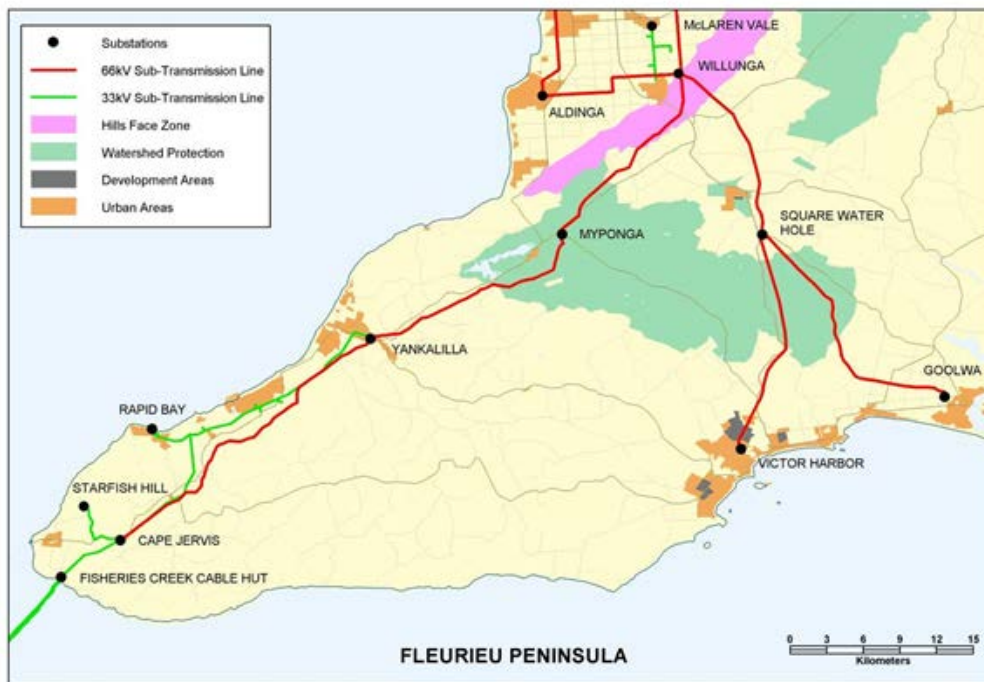
Figure 2-1 Current Fleurieu Peninsula Electricity Network
