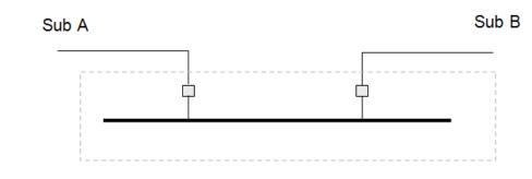
Step 3.2: The stand-alone arrangement for the provision of *prescribed common transmission services* to an equivalent standard is shown below and consists of 3 circuit breakers.
