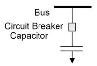
Branch with Capacitor, Circuit Breaker and Bus
