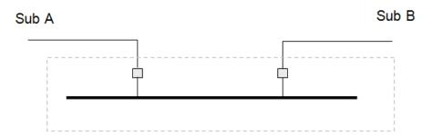
Step 3.2: The stand-alone arrangement for the provision of *prescribed common transmission* services to an equivalent standard is shown below and consists of 3 circuit breakers.
