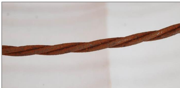
FIGURE 2 - CORRODED 3/0.104 SC/GC CONDUCTOR
