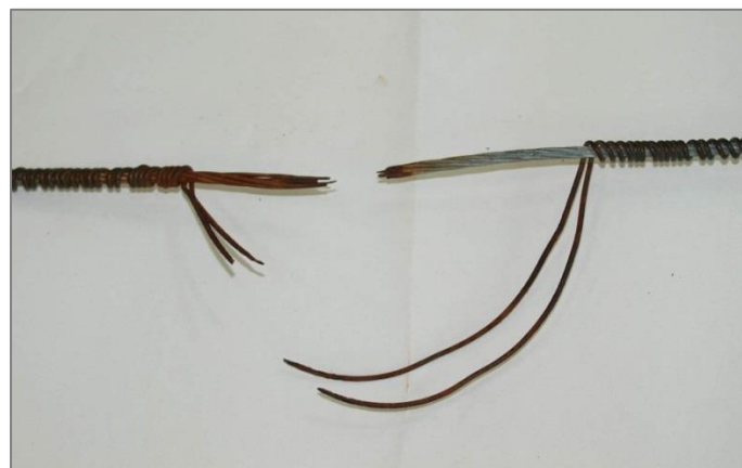
FIGURE 3 - FAILED 7/0.064 SC/GZ CONDUCTOR
