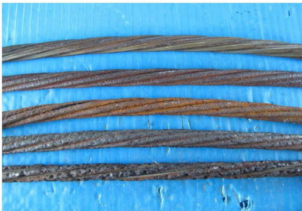
FIGURE 4 – VISUAL COMPARISON OF CONDUCTOR CORROSION CATEGORIES
