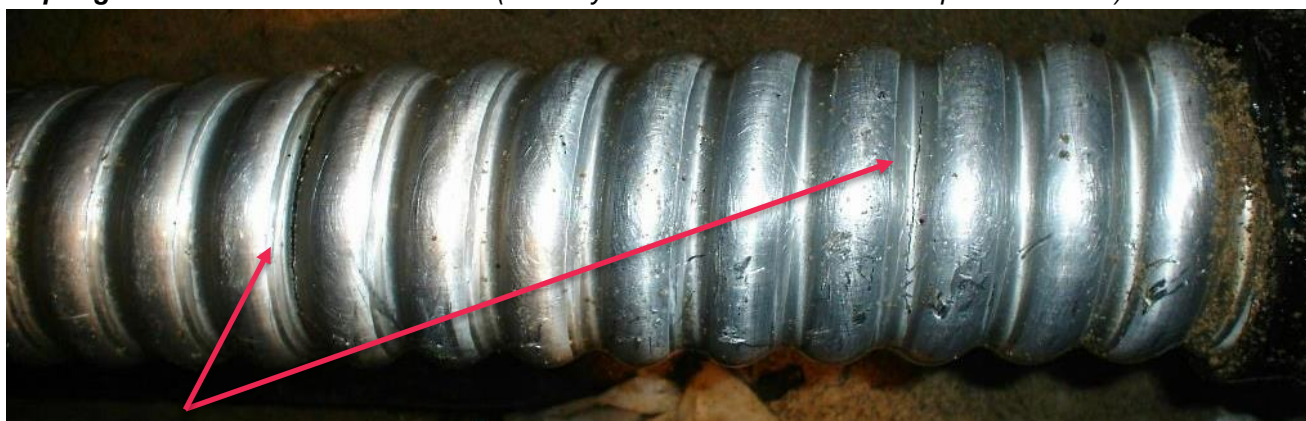
Middle – Feeder 233 sheath (existing cracks around sheath and additional cracks forming) - 2011
