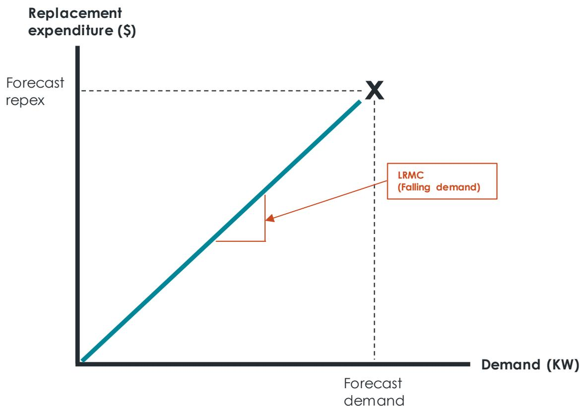
Our analysis indicates that this ‘linear’ assumption would lead to an estimate of LRMC equal to \$73/kW for the low voltage tariff class. However, our discussions with network planning engineers indicated that an assumed linear relationship would significantly overstate the effect of a fall in demand on replacement expenditure.
