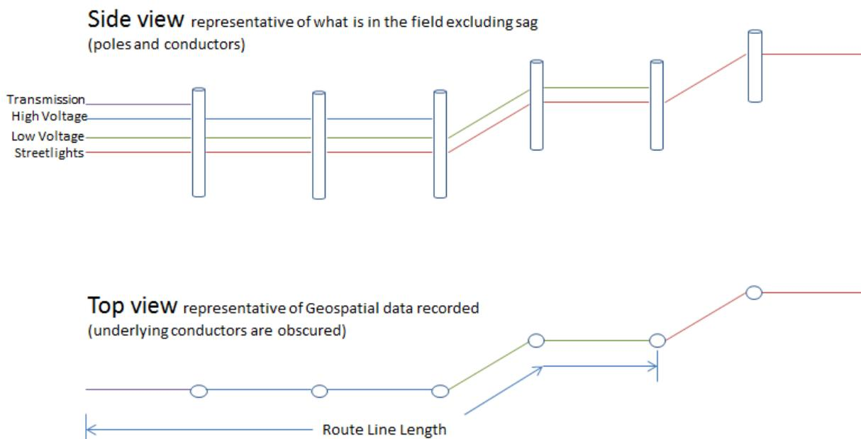
Route Line Length effectively based on single route length as shown by the top view (excluding service lines to customers, public lighting, communication and similar service or pilot lines). Endeavours' geospatial system captures overhead lines as point to point data and does not include components such as sag, etc.
