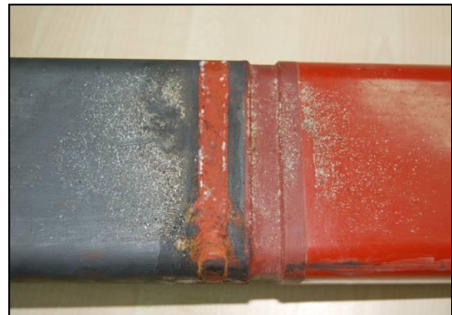
SSCVL Close up of earth screen damage
