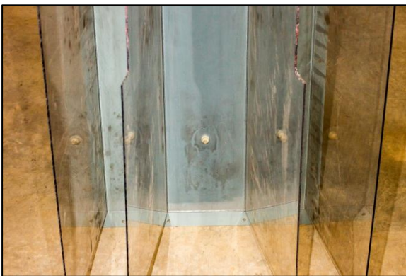
PD on nylon screws SSLYT CB1022
