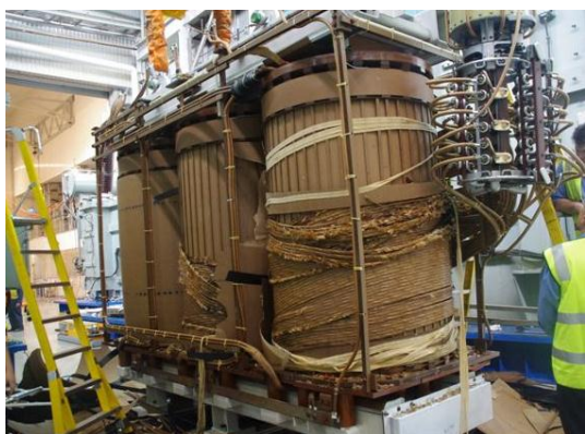
Figure 14: 110/33kV Transformer winding damage after a fault and corresponding waveform capture from the protection relay disconnecting the fault in 120ms.
