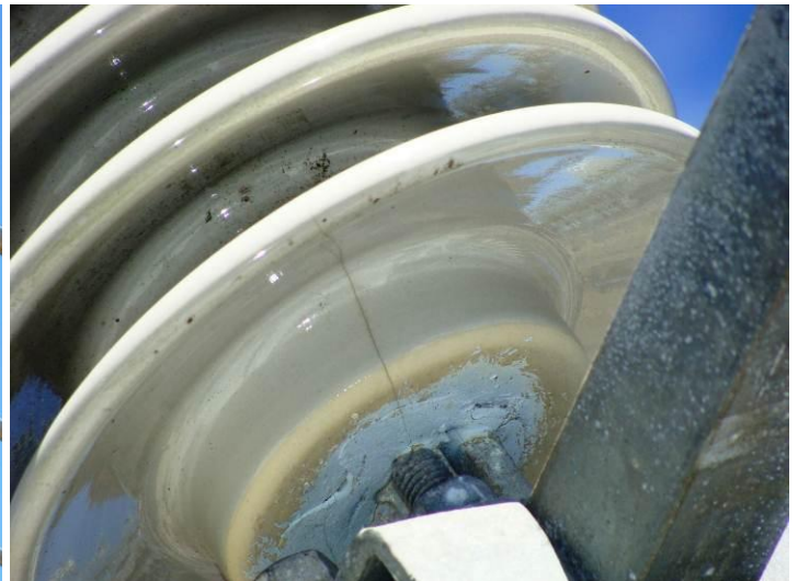
Fig 1- A typical 33 kV [REDACTED] isolator in switchyard Figure 2- Hairline crack on the support insulator.
