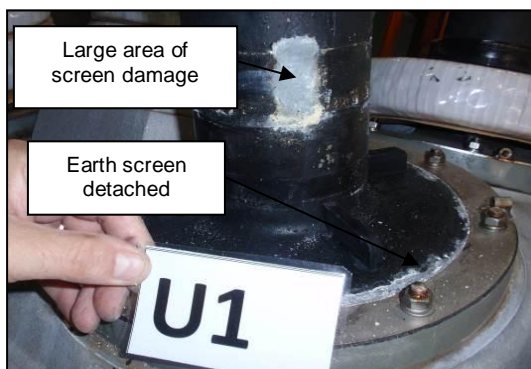
SSDRA CB3T22 screen degradation
