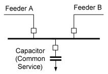
Step 3.2: The stand-alone arrangement for the provision of *prescribed common transmission services* to an equivalent standard is shown below and consists of 3 circuit breakers.
