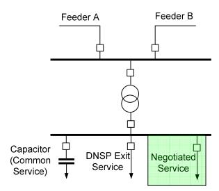
Step 1: The branches are Feeder A, Feeder B, DNSP Exit, Tie Transformer and Capacitor, the negotiated service branch is not considered as discussed above.
