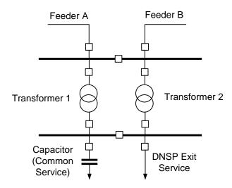
Step 1: The branches are Feeder A, Feeder B, DNSP Exit, Transformer 1, Transformer 2 and Capacitor.
