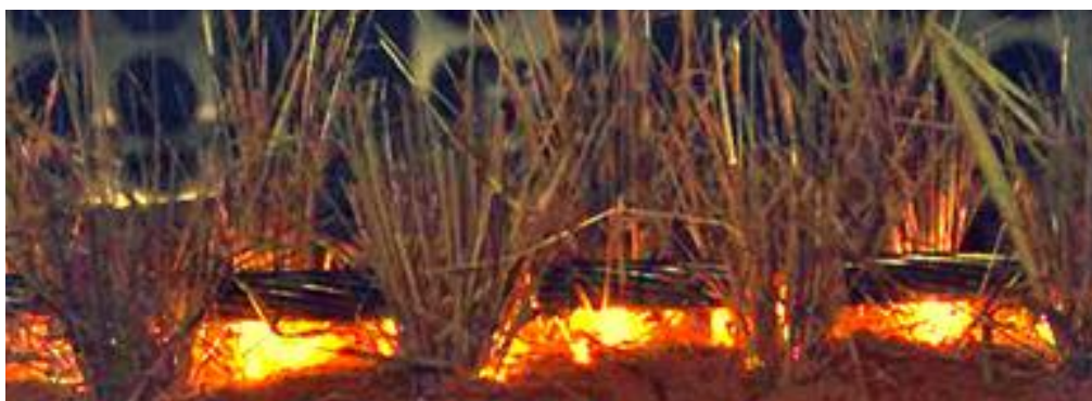
Distribution of conductor-soil arcs at instant of initial contact (16 amps, 19/3.25AAC conductor) 25
