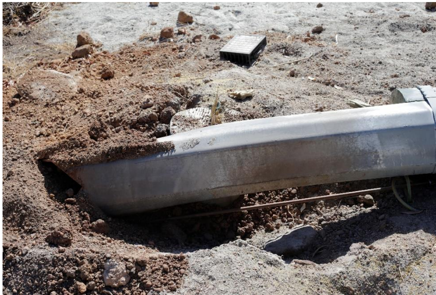
Figure 15: Example of a foundation failure of a banded reinforcement type.
