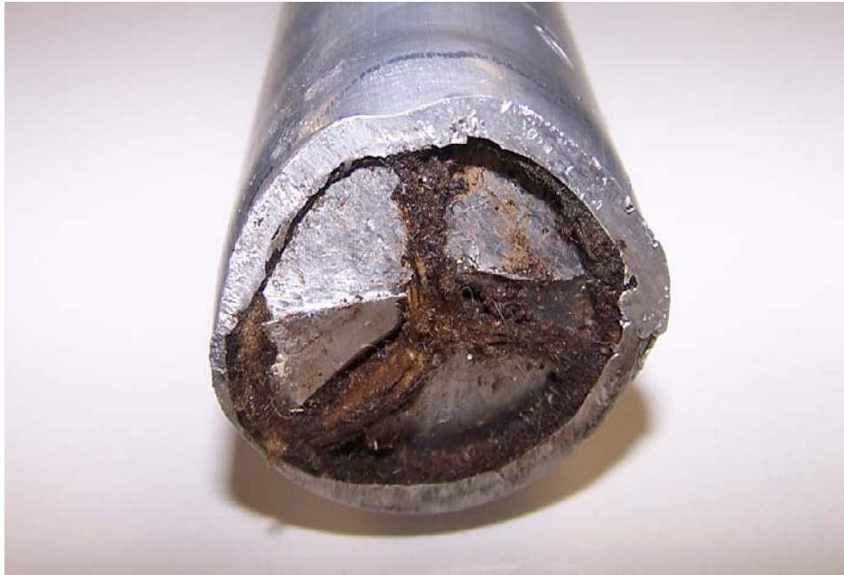
Figure 6 – A section of CONSAC showing deteriorated paper insulation (caused by moisture ingress)
