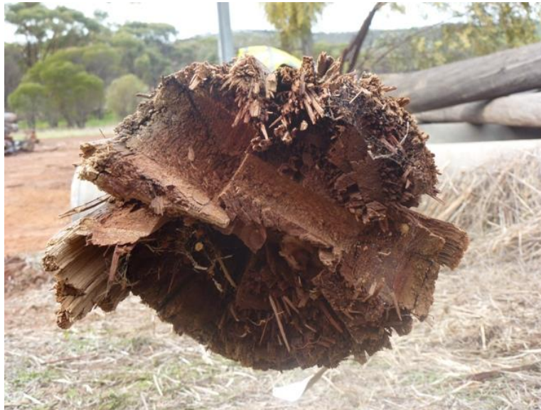
Figure 10: Failed section of pole through the top bolt & ferrule hole. This would lead to a 9-42% loss of strength depending on the orientation of the bolt hole.
