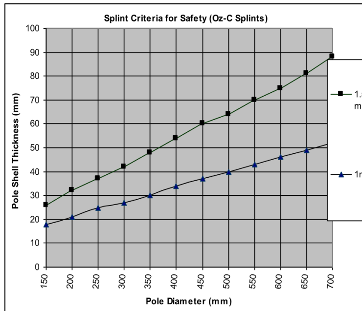
Figure 4: Minimum wall thickness criteria at the top of the splint for C-Splint reinforcement.
