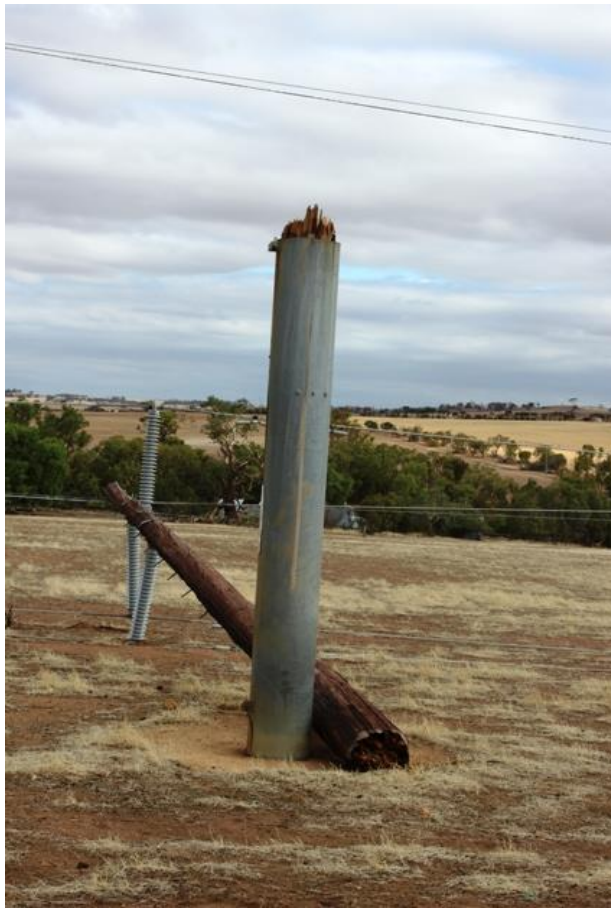
Figure 16: Failed rebutt pole at the timber-steel interface due to timber decay and high winds.
