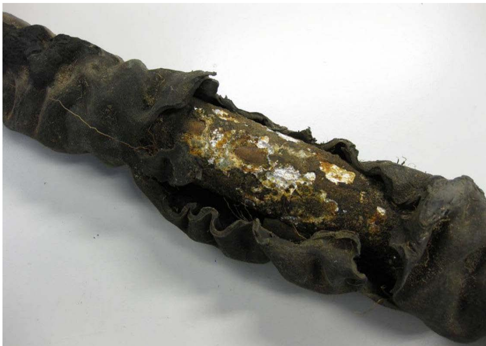
Figure 5 – A section of CONSAC showing corroded aluminium sheath
