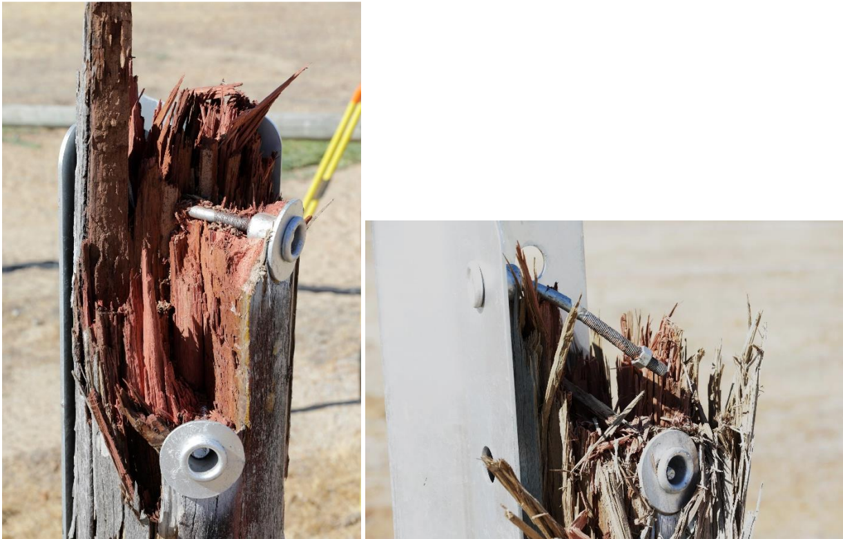
Figure 12: Examples of failures being influenced by both top bolts. The top bolt in the right hand image also pulled through the ferrule during failure.
