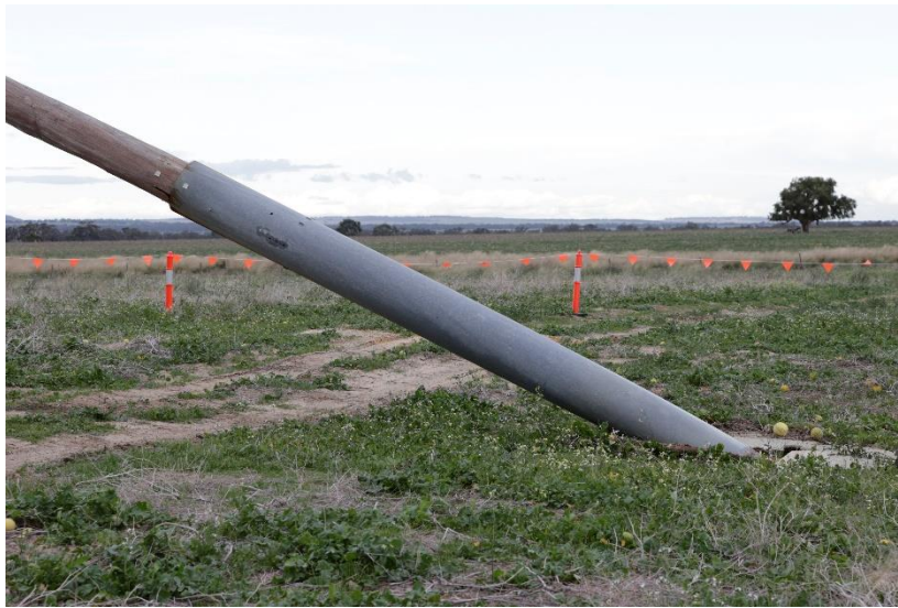
Figure 17: Failed rebutt pole at ground line due to steel section buckling.
