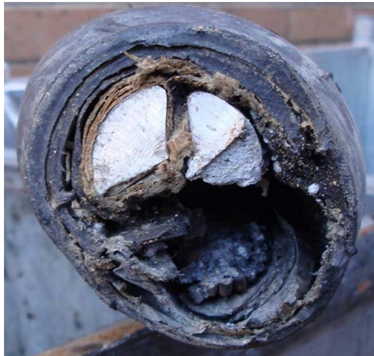
Figure 7 – A section of CONSAC showing a failed joint
