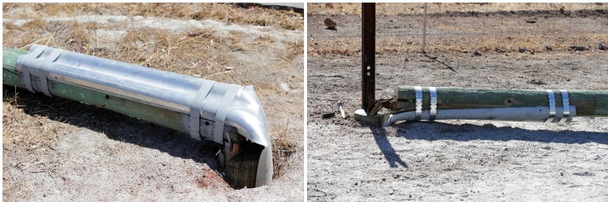
Figure 7: Examples of banded reinforcement failure about the weak axes.
