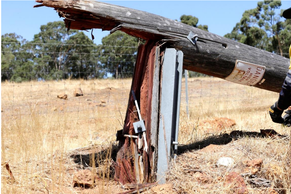
Figure 14: Example of a barber-chair failure for bolted reinforcement.
