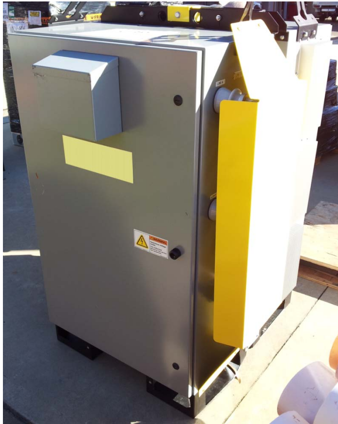
Figure 11 - Low Voltage Regulator
