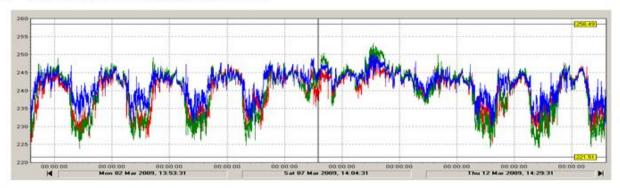
AFTER – voltage range 248V to 234V, unbalance 5V Normal voltage fluctuations still apparent away from 245V and 239V reactive power support levels
