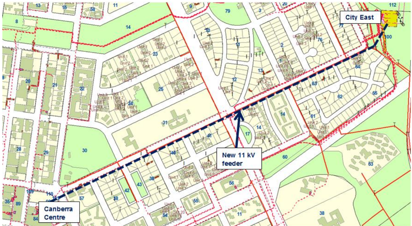
Figure 1: Proposed 11 kV feeder cable route City East Zone Substation to Canberra City
