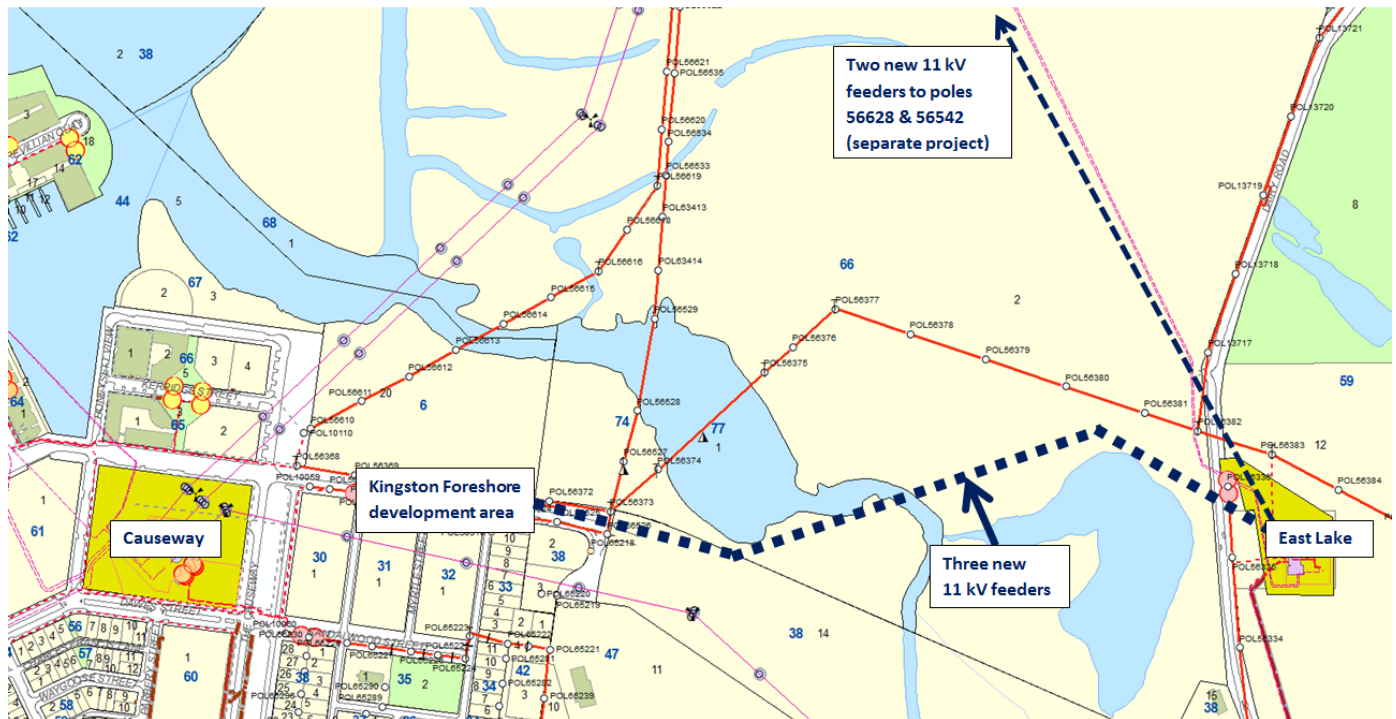
Figure 7: Proposed 11 kV feeder cable route East Lake Zone Substation to Kingston Foreshore
