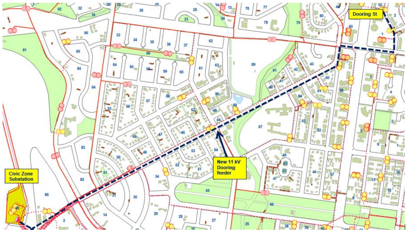
Figure 2: Proposed 11 kV feeder cable route from Civic Zone Substation to Dooring St
