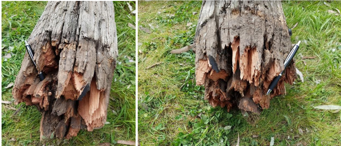
Figure 4 Failed Pole, Otherwise solid, but for drill holes and advanced decay
