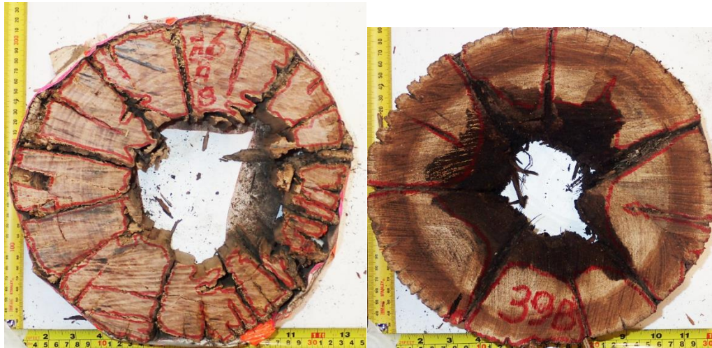
Figure 3 Decayed Pole Cross Section
